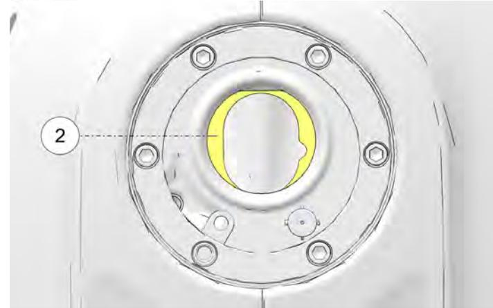
2. Insert the fuel nozzle into the fuel tank filler neck.
